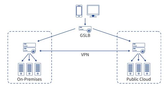
Figure 1- LoadMaster Hybrid Topology
